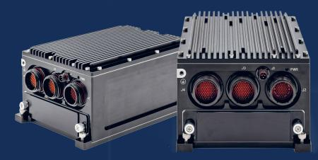
Powered by the latest generation of Intel® processors and MIL-GRADE qualified. The computer is manufactured in Europe and is a highly integrated processing system ready for deployments in extreme environments.
